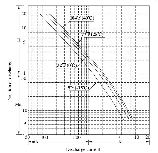
**Constant Current Discharge Rating Amperes @ 77°F (25°C)**
